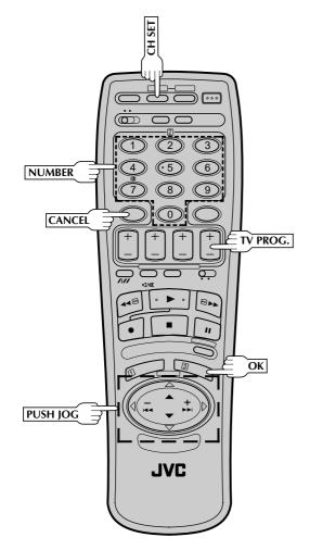
With Video Plus+, timer programming is greatly simplified because each TV programme has a corresponding code number which your recorder is able to recognize.
